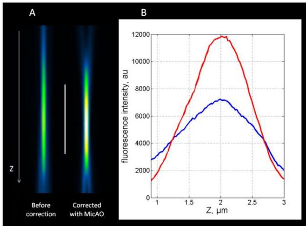
**Figure 2.** The Z profile of the 200nm fluorescent bead at 22µm depth in 2% agarose. A. Before and after correction of aberrations. The size of the scalebar is 1µm; B. The intensity profile along the Z axis before (blue) and after (red) correction of aberrations. The size of the scalebar is 1µm.
