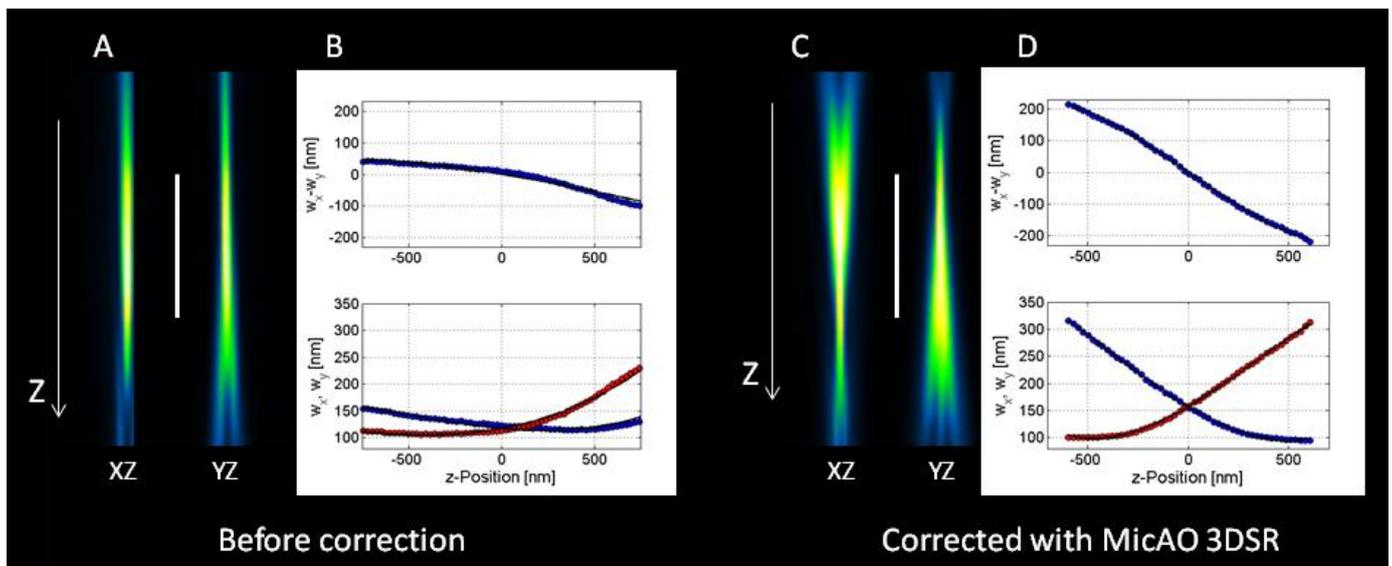
**Figure 3.** The effect of correction of aberrations at 22µm depth in 2% agarose. A. The XZ and YZ projections of the PSF with applied 90nm RMS of astigmatism before correction of aberrations; B. The calibration curve before the correction; C. The XZ and YZ projections of the PSF with applied 90nm RMS of astigmatism after correction of aberrations with MicAO 3DSR; D. The calibration curve after the correction. The size of the scalebar is 1µm.
