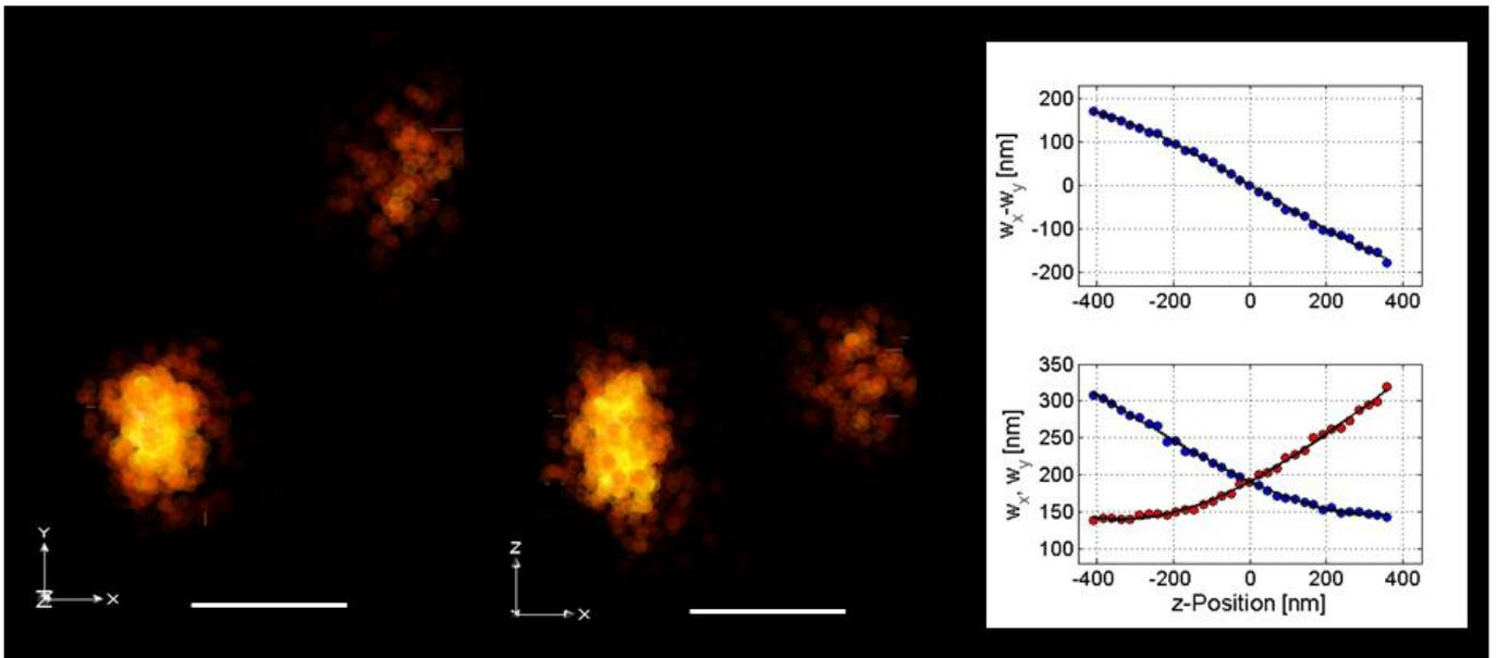
**Figure 4.** Two projections of mEos2 labeled Centrin1 at 50µm depth in 2% agarose imaged with 3D PALM. The amount of astigmatism induced on the deformable mirror during the imaging was 130nm RMS. The scale bar is 200 nm. For visualization of results we used ViSP software (El Beheiry and Dahan, 2013).
