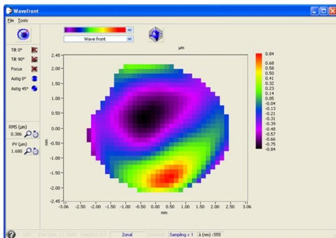
Figure 4 - Uncorrected: RMS: 0.386µm, PV: 1.680µm
