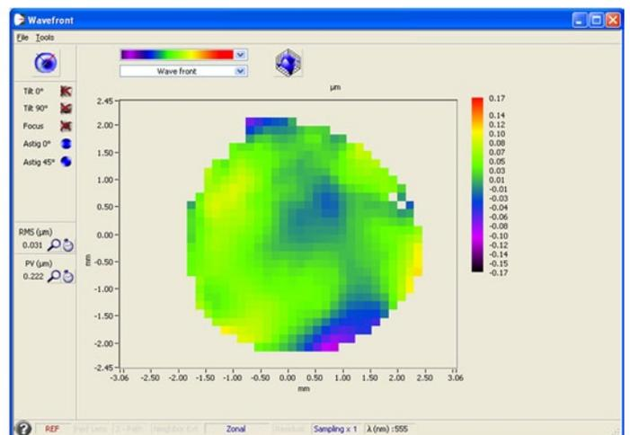
Figure 5 - Corrected: RMS: 0.031µm, PV: 0.222µm
