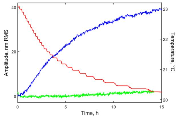
**Figure 3.** Ambient temperature dependence of the wavefront without (blue) and with (green) stabilization module installed on the deformable mirror. Temperature change is shown in red.
