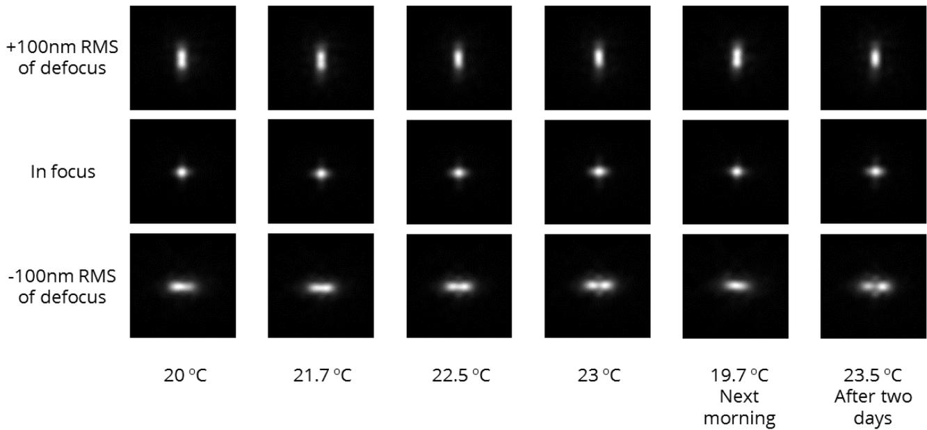
**Figure 4.** Example images of the diffraction-limited fluorescent bead at different ambient temperature. The 60nm RMS of astigmatism was added using the deformable mirror. Middle row – the bead is in focus, the upper and lower rows – the bead is slightly out of focus.
