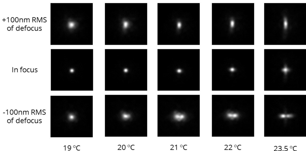
**Figure 1.** Example images of the diffraction-limited fluorescent bead at different ambient temperatures without stabilization module inside MicAO. Middle row - the bead is in focus, the upper and lower rows - the bead is slightly out of focus.
