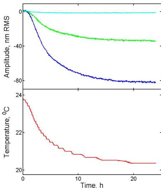
**Figure 2.** Ambient temperature dependence of various Zernike modes without active control on the deformable mirror (upper panel); astigmatism 0 (blue), astigmatism 45 (green) and 3<sup>rd</sup> order spherical aberration (cyan). Temperature variation is shown in red on the lower panel.
