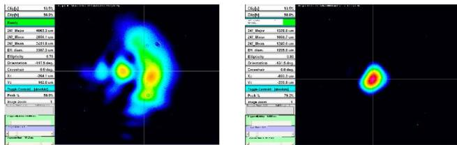
**Figure 6.** Beam profile: left - uncorrected, right - corrected.
