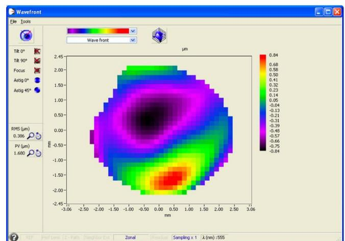
**Figure 4.** Before correction: RMS  $0.386 \mu\text{m}$ , PV:  $1.680 \mu\text{m}$
