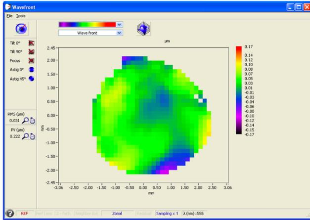
**Figure 5.** After correction: RMS 0.031  $\mu\text{m}$ , PV: 0.222  $\mu\text{m}$
