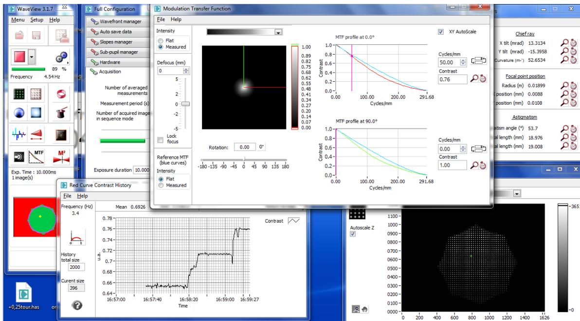
Figure 6 Screen shot of the MTF measurement.
