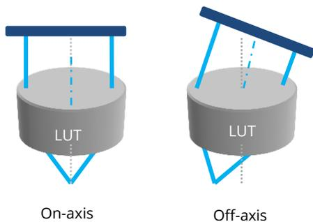
**Figure 3** Schematic of on- and off-axis measurements.
