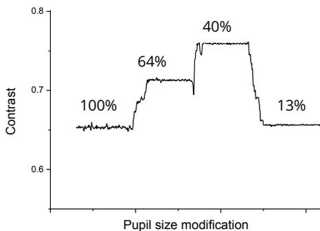
Figure 7 Change of the MTF contrast as a function of diaphragm aperture in percent.
