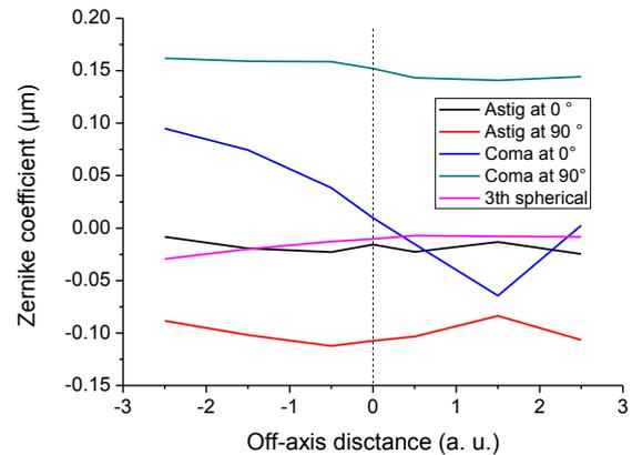
**Figure 5** Zernike coefficients at different off-axis positions.
