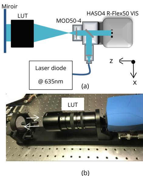
**Figure 1** (a) Schematic of the optical setup with HASO4 R-Flex50, objective module MOD50-4, lens under test (LUT) and a plane mirror, (b) a photograph of the setup for the camera lens test using auto-collimation.
