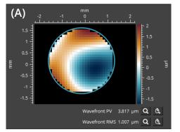
Target wavefront is  $1.007 \mu m$  RMS (combination of Zernike polynomials up to the 4th order)
