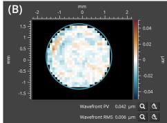
Wavefront error in closed-loop WFE = 6 nm RMS
