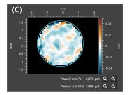
Wavefront error in open-loop WFE = 9 nm RMS
