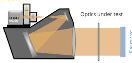
The R-Flex 2 SWIR Large Aperture is a combination of the HASO R-Flex SWIR and a beam collimator for the measurement of large optics in the 1.0-1.7  $\mu m$  wavelength range. It is suitable for flat window, windshield, plane mirror and laser beam analysis. Possible aperture sizes are from 30 mm up to 150 mm.
