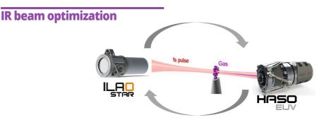
IR phase aberrations are transferred to the generated EUV beam. Correcting the femtosecond wavefront is therefore crucial. Imagine Optic provides adaptive optics systems including HASO wavefront sensor and ILAO Star deformable mirror to optimize the driving beam, and EUV wavefront sensor for easy phase characterization and shaping.
