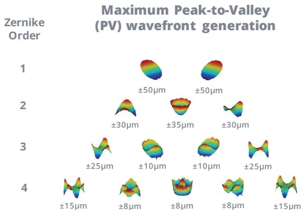
RMS residual wavefront error : max 0.02µm (generation of Zernike mode of the order <5 with amplitude set at 20% of the total dynamic range)
