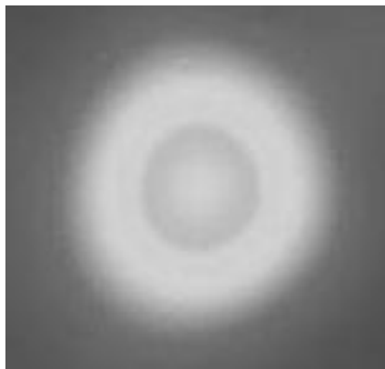
Fig. 11. Focal spot in the experimental chamber. A 50 mm beam is focused by a 1 m parabola. The size is 1.3 times the diffraction limit but the Strehl ratio is only 40%
