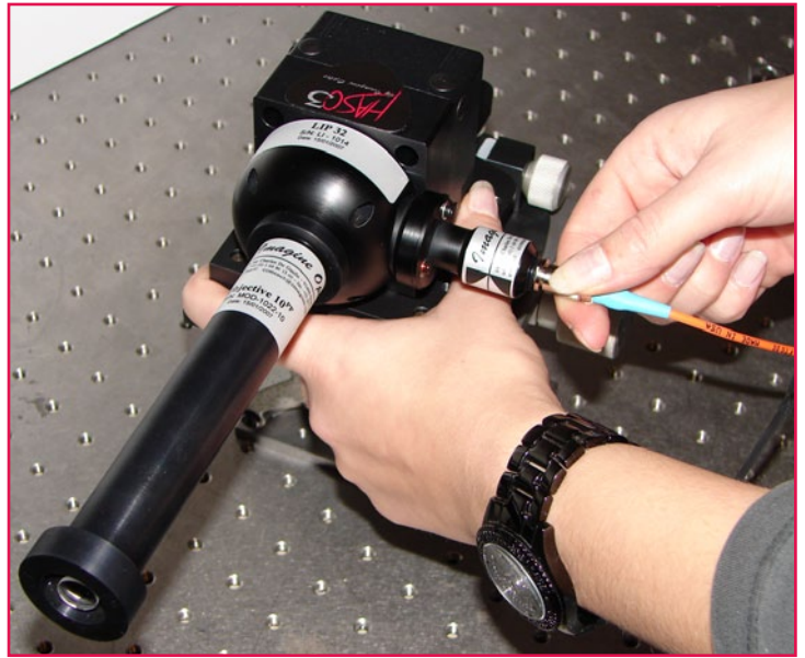
Laser Diode (included with all models) being attached to a HASO R-Flex 32 with an f/10 objective.
